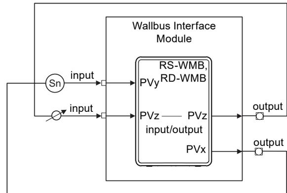
This can be seen in the diagram where PVx is the output from the RD-WMB which is connected to a sensor module in the strategy. The sensor's output is then sent back to the RD-WMB for display (PVy). This enables the strategy to change the value before display (e.g apply an offset).
