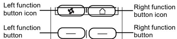
In the normal configuration shown above, the left button will select manual fan control, and the right button, manual occupation override.
