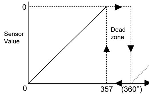
This helps to prevent spikes on Trend plots of the direction when the wind is northerly. The decision whether to set the value to 0 or 357 is made by F4 and F5. F2 detects when the direction is in the dead zone by looking for a value of S that is less than 4V, and if it finds that this is the case it switches the output of F5 through Gate F3, rather than the direction calculated by F6.
