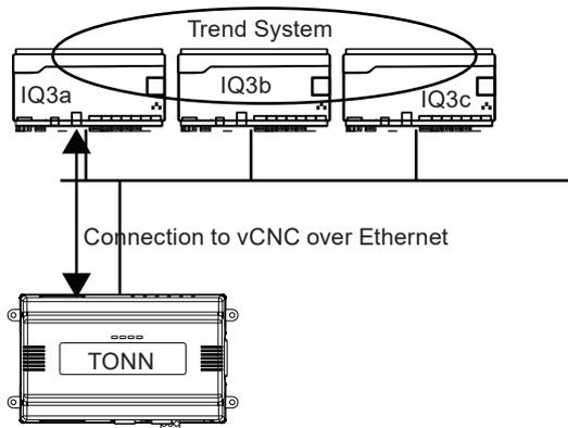
In the diagram above the TONN is connected to the IQ System over Ethernet using a vCNC in IQ3a. It is able to discover the Trend system including available values (IQ3a, IQ3b, and IQ3c).
